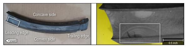
Figure 7. Fatigue indications on fan blade fracture surface.
