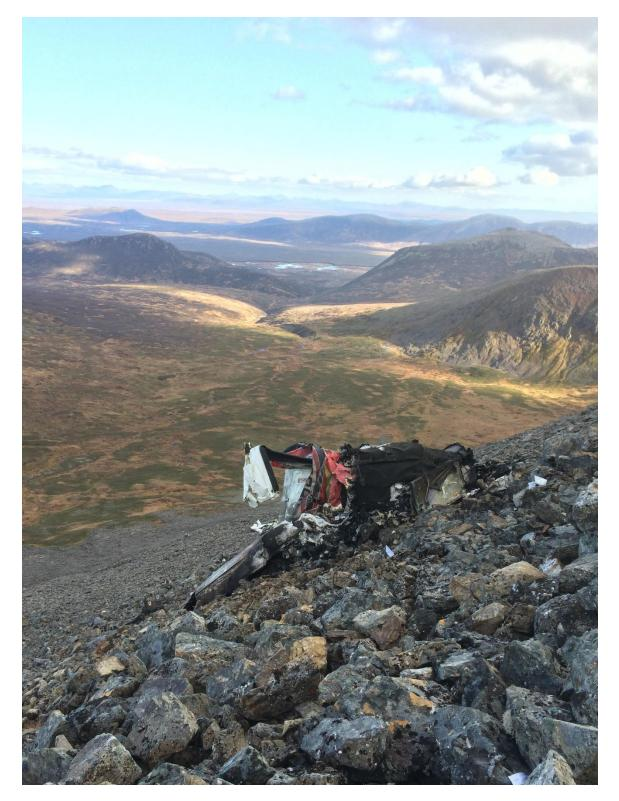
Figure 6. Separated section of empennage with vertical and horizontal stabilizers and rudder attached.
