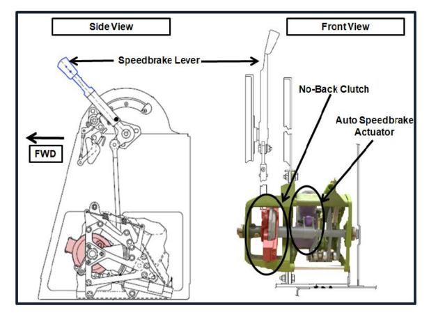
**Figure 4.** Two diagrams showing the cockpit center console, the speedbrake lever and its linkages, and components of the automatic speedbrake system. The no-back clutch mechanism has been highlighted in the side view diagram on the left. A photograph of the speedbrake actuator and no-back clutch mechanisms has been superimposed on the front view to show those components' relative positions within the center console.
