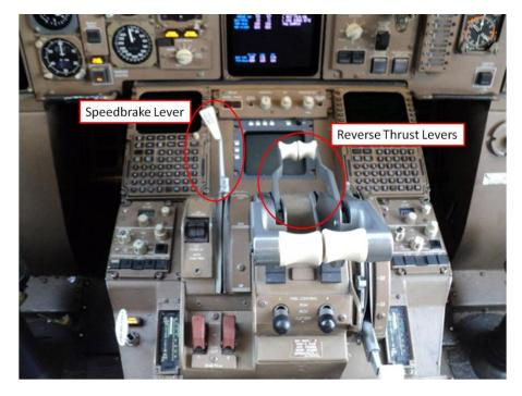
**Figure 3.** A photograph of the center console in the incident airplane's cockpit, with the reverse thrust lever and speedbrake levers marked.
