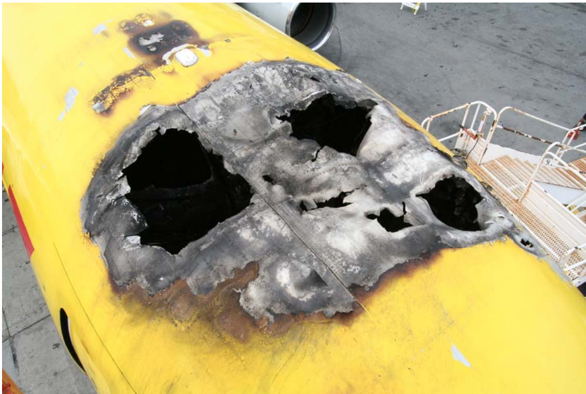
Figure 2. Fire Damage to Top of Airplane
