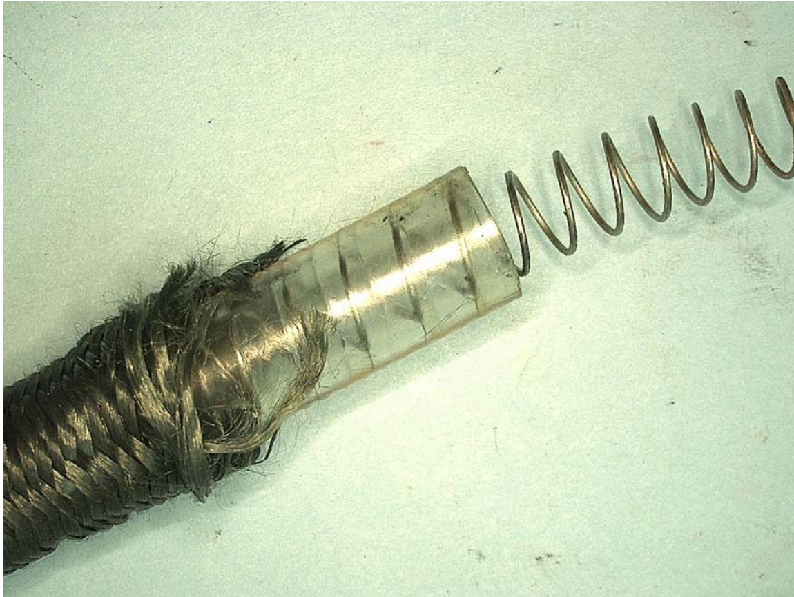
Figure 4. Stainless Steel Coil Spring Within Flexible Oxygen Hose
