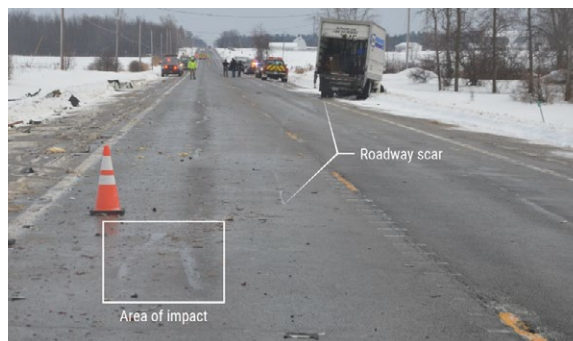
FIGURE 16. Eastbound SR-37 showing area of impact and roadway scar extending to truck's damaged left front wheel assembly.
