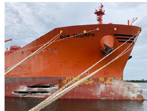
FIGURE 31. Bow Triumph at the Odfjell Terminal in Charleston on September 8, 2022, showing damage to the vessel's starboard side. SOURCE: US COAST GUARD
