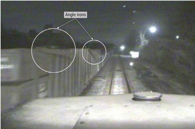
FIGURE 41. Gondola car and protruding angle iron section immediately before impact. SOURCE: NORFOLK SOUTHERN RAILWAY, ANNOTATED BY NTSB
