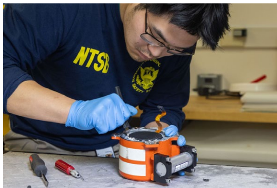
FIGURE 22. Vehicle Recorder Division staff member examining a cockpit voice recorder recovered from the PSA Airlines Bombardier CRJ700 following the midair collision with a Sikorsky UH-60 military helicopter near DCA in Washington, DC.
