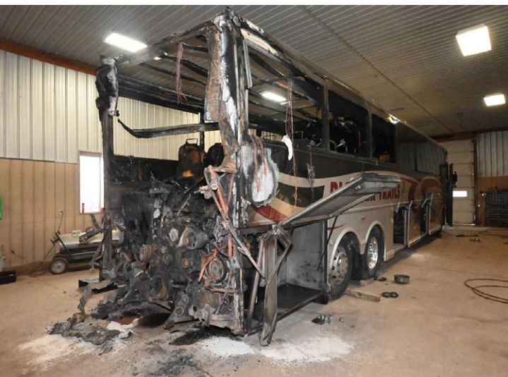
FIGURE 10. Damage to right rear of motorcoach from crash and postcrash fire.
