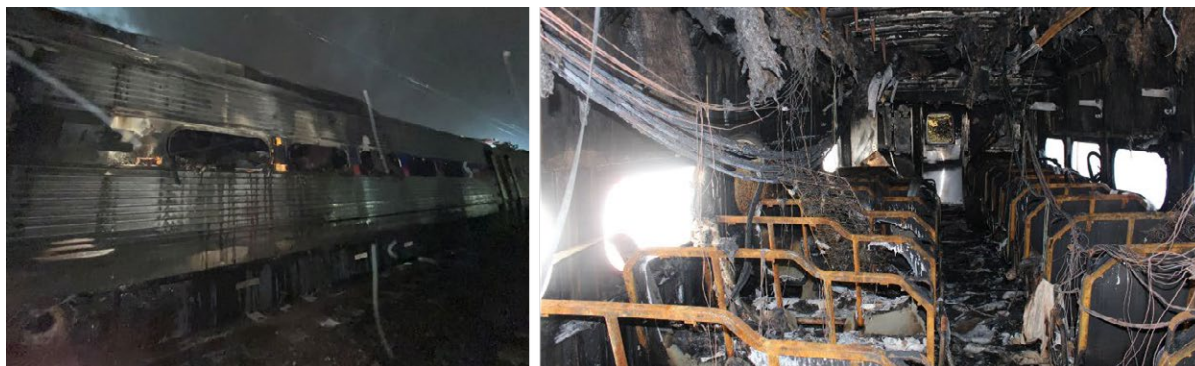
FIGURE 17. From left: Exterior and interior views of fire damage to a SEPTA Silverliner IV railcar. SOURCE (LEFT): SEPTA.
