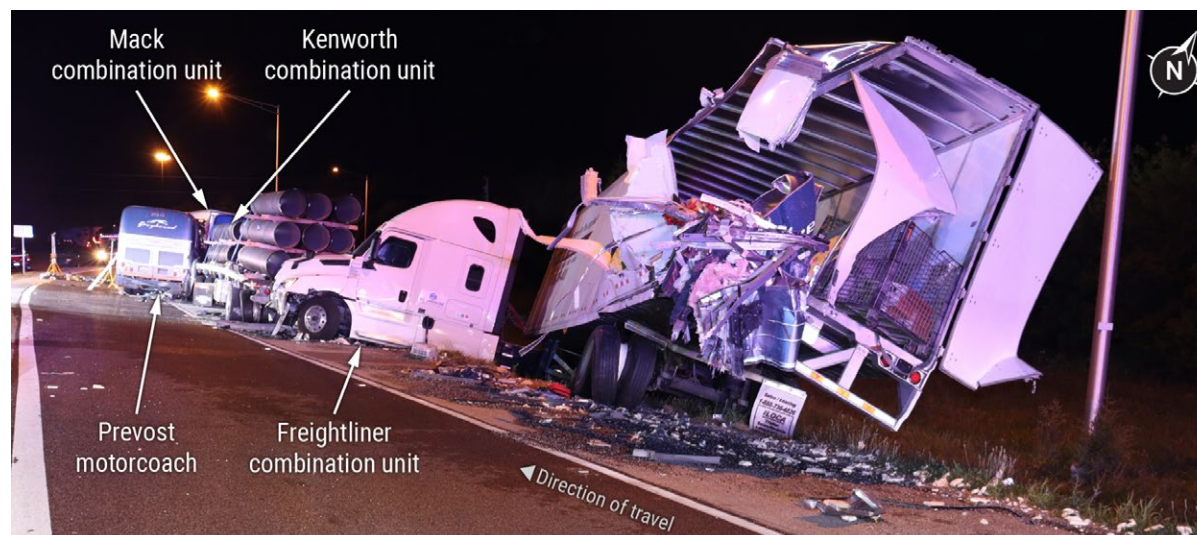
FIGURE 11. Crash scene showing the motorcoach (Prevost) and three tractor-trailer combination vehicles (Mack, Kenworth, and Freightliner) positioned along the roadway following the collision.
