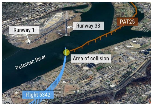
FIGURE 6. Preliminary ADS-B flight track for flight 5342 (blue) and preliminary radar data for PAT25 (orange).
