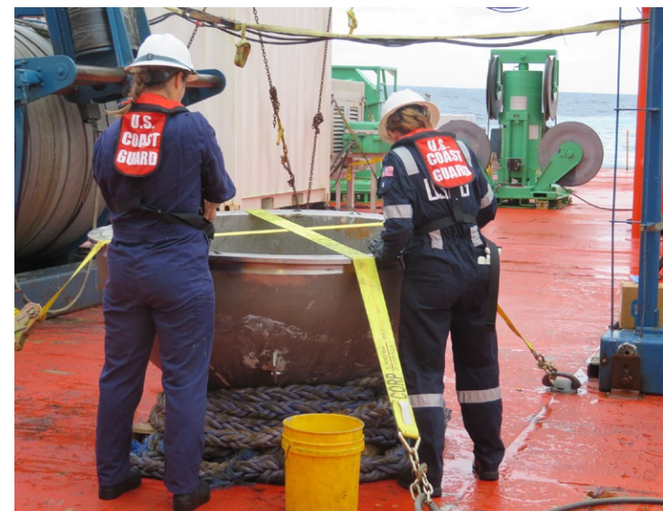
Coast Guard marine safety engineers examine the aft titanium dome from the Titan on October 1, 2023, in the North Atlantic Ocean. The dome was recovered from the seafloor and transferred to a US port for analysis.
