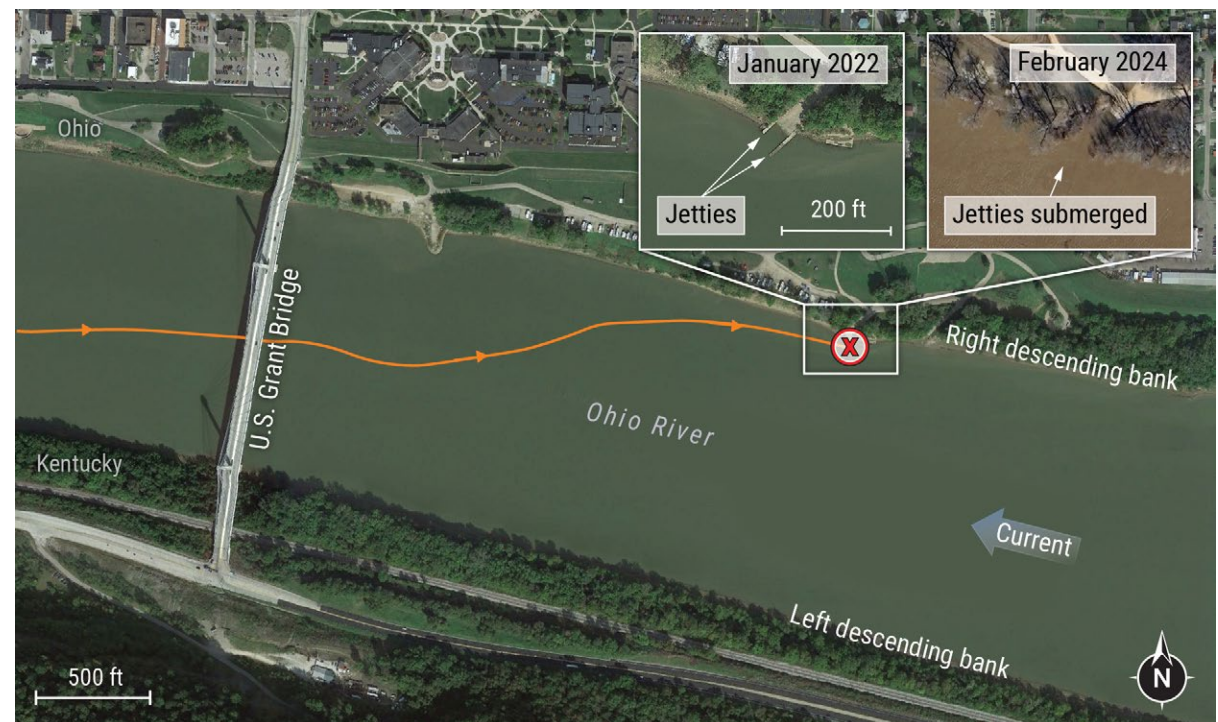
Trackline of Tom Frazier tow as the vessel transited through the U.S. Grant Bridge and toward the right descending bank. Inset satellite photos show the jetties visible on January 26, 2022 (17.4 to 18.5 feet at the Portsmouth gage) and submerged on February 14, 2024 (28.7 to 31.6 feet at the Portsmouth gage).
