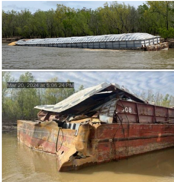
From top: Covered barge LTD 4611 partially sunken by its bow to port, and damage to the stern area of MTC 500B, the barge that was immediately aft of the PTC 706.
