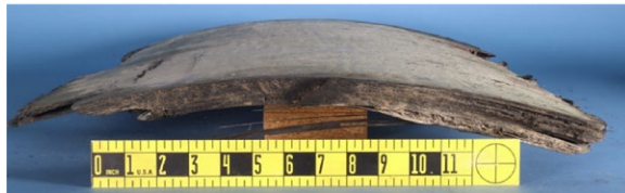
From top: Recovered carbon fiber composite cylinder machined end face, and mid-span fractured face.
