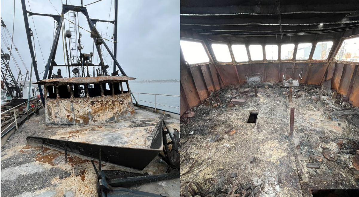
Fire damage to the foredeck of the Three Girls and the interior of wheelhouse.
