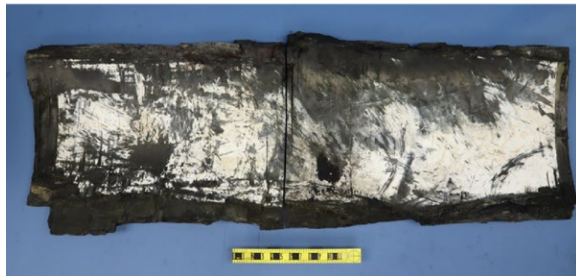
From top: Recovered carbon fiber composite pressure hull outer surface and inner surface.
