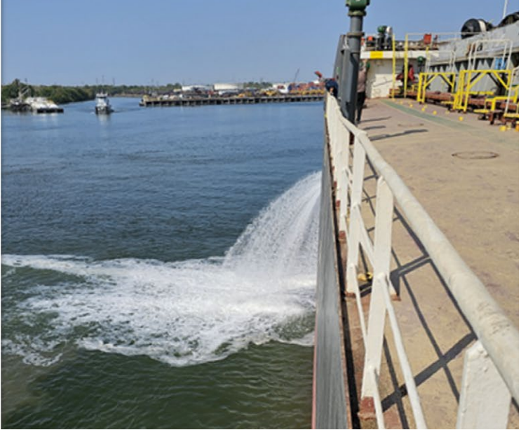
BBC Africa and Common Faith after the collision and ballast water spilling from Common Faith punctured port ballast tank (circled at left). SOURCE: COMMON FAITH MASTER.
