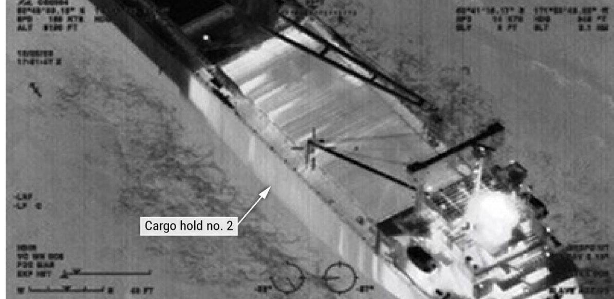
Infrared photo of the Genius Star XI en route to Dutch Harbor, showing an indication of heat (in white) within cargo hold no. 2 on December 28. BACKGROUND SOURCE: COAST GUARD.
