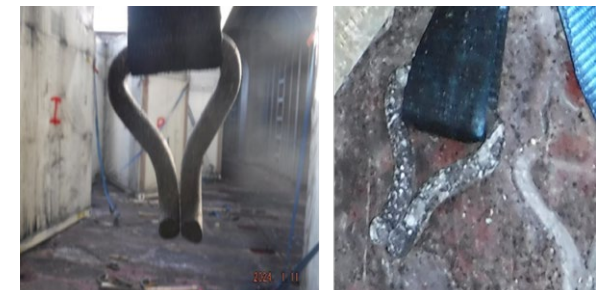
Two separate hooks that fractured and separated from a D-ring. SOURCE: COAST GUARD.
