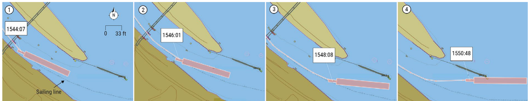
The Amber Brittany tow as it came through the Louisville and Indiana Railroad Bridge, its heading altered to port, it was set off the sailing line, and it contacted the vane dike mooring cell.
