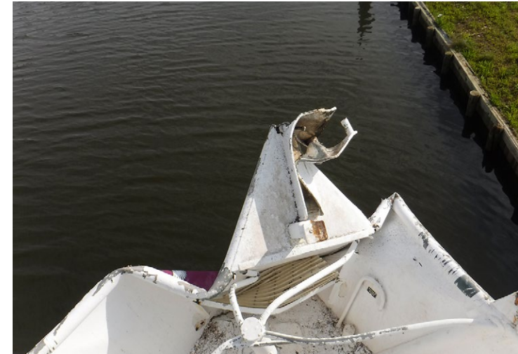
Damage to Papa Rod 's bow. SOURCE: COAST GUARD.
