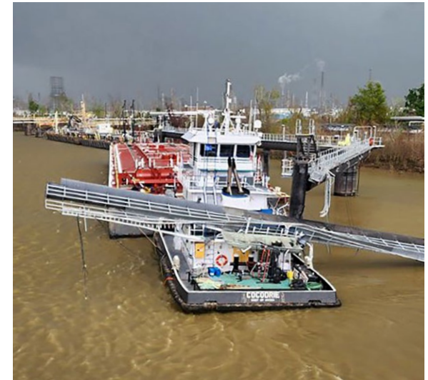
Cocodrie with the walkway resting across the deck of the aft main deck structure. SOURCE: COAST GUARD.
