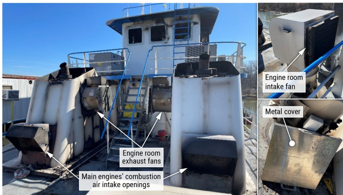
Johnny M exhaust stacks showing covered engine room exhaust fans and engine air intake openings (two openings under each hood). Insets, from top: Engine room intake fan (there were two intake fans—one port and one starboard) and metal cover, all located on upper deck.
