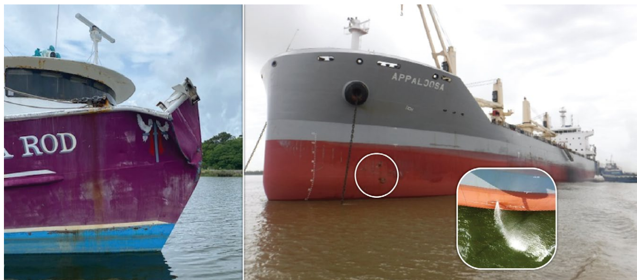
Bow damage to the Papa Rod and Appaloosa hull breach (circled). Inset shows ballast water leaking from the breached hull. SOURCE: COAST GUARD.
