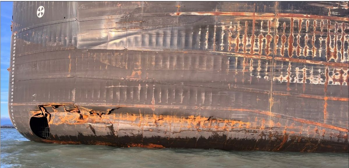
Damage to the port side of the American Mariner after striking the Munuscong Channel Junction Light.
