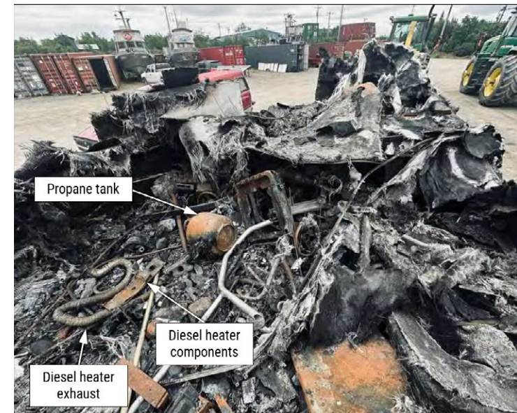
Fire damage to the Jordyn Rose bow (facing forward).
