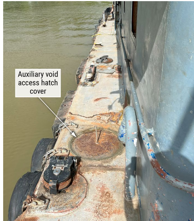
Cajole after the sinking, with starboard-side auxiliary void access hatch cover replaced and permanently sealed to the main deck for transit to shipyard.
