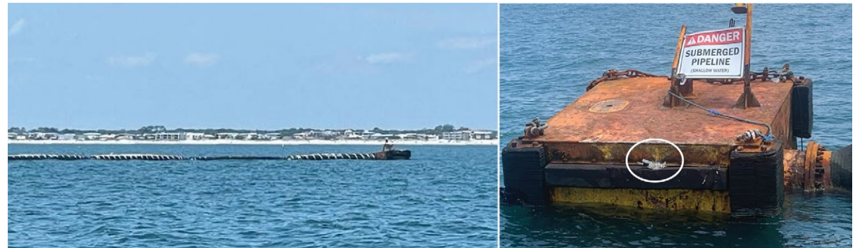
From left: The dredge pipeline pump-out cube and floating hose from a distance, after the casualty. The pump-out cube with damaged sign and the area where the Atlantis made contact (circled).
