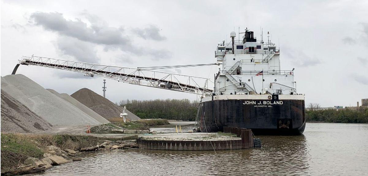
John J Boland discharging cargo using its self-unloading boom in Lorain, Ohio, after the grounding.
