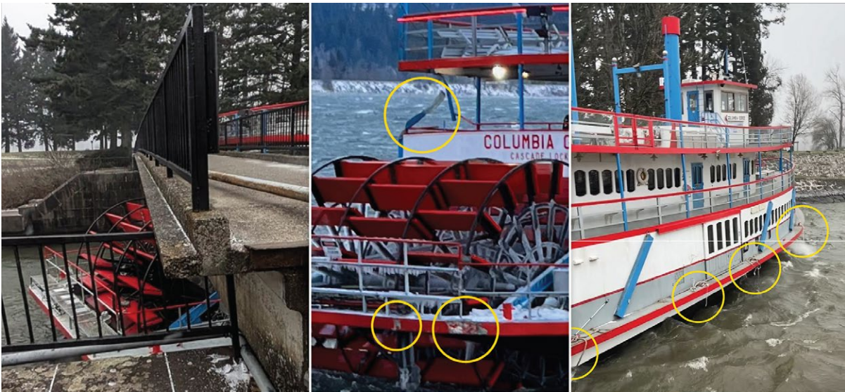
Left to right: The stern of the Columbia Gorge under the Thunder Island pedestrian bridge as seen from the mainland; damage to the stern and the support columns for the upper deck of the Columbia Gorge (circled); and the vessel in the lock with broken moorings visible (circled). BACKGROUND SOURCE: JETTYLIGHT LLC.
