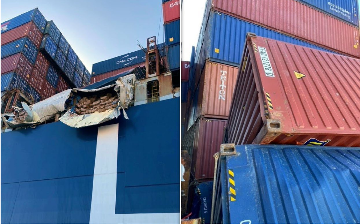
Area of the container collapse in bay 42 on the port side of the President Eisenhower and closer view of the collapsed containers. SOURCE: COAST GUARD.
