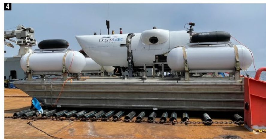
Simplified representations of the Titan (scale approximate). 1: Outboard profile. 2: Inboard profile (pressure hull area highlighted in gray). 3: Plan view of Titan on LARS. 4: Titan secured on LARS in 2022. SOURCE (4): GARRY COMBER.
