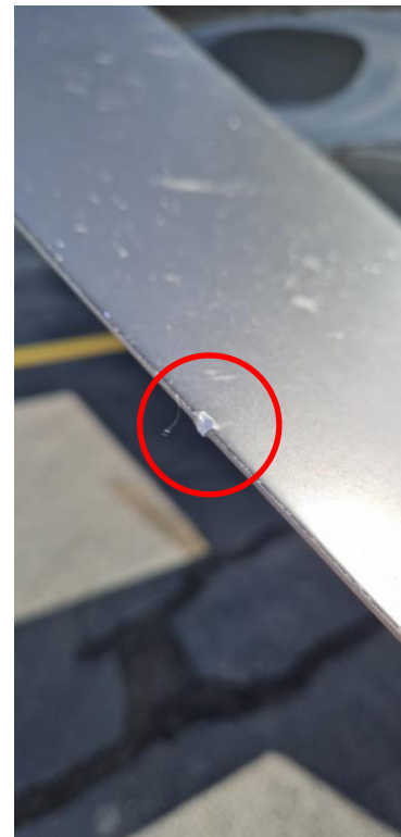
Figure 1. Nick in aluminum propeller blade. (Source: Hartzell Propellers)
