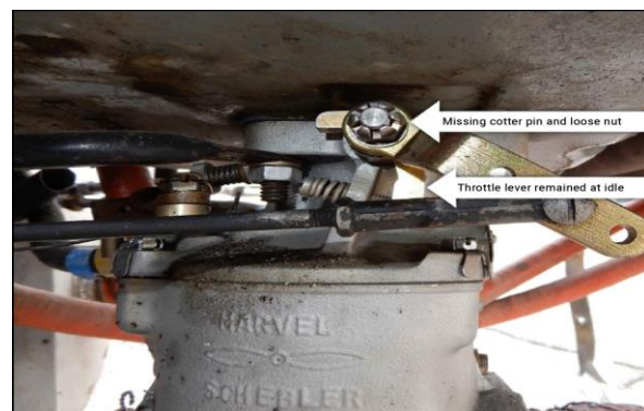
Figure 2. Missing cotter pin and unsecured throttle lever locking nut.
