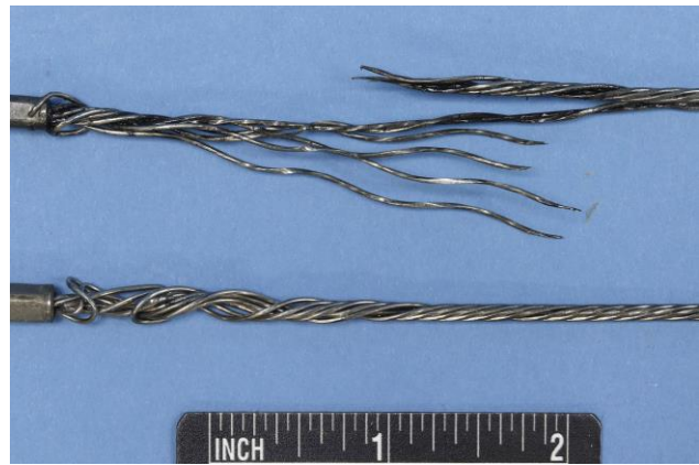
Figure 1. Worn throttle cables in need of replacement.
