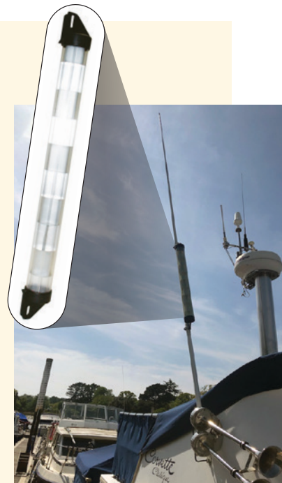
Figure 2. Above and right: Exemplar radar reflectors mounted on small vessels.
