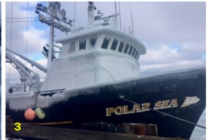
Ice accumulation on a vessel operating near the capsized vessel that was lost with all hands in the Bering Sea on February 11, 2017. (1, 2, and 3) *Polar Sea*: ice covers the decks and anchor chain during the vessel's transit to St. Paul Island on February 10 and remains on the wheelhouse while it was docked at the island the following day.
