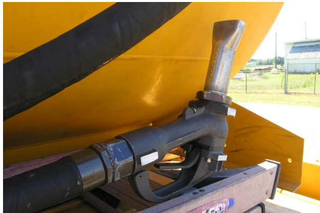
Figure 2. Photograph of Jet A fuel nozzle.
