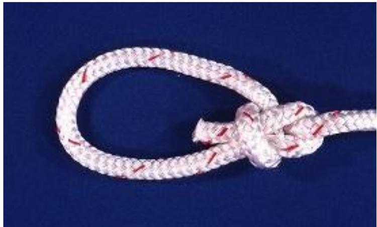
**A bowline knot, the knot most commonly used by parasailing operators in their towlines. This type of knot can weaken a brand-new rope by as much as 70 percent.**
