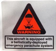
If a parachute deployed and is still attached to the airplane, **do not enter the airplane until the parachute is fully collapsed**, as it could reopen, catch the wind, and drag the airplane.
