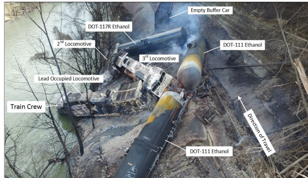
Figure 24. Aerial view following the CSX Transportation derailment with hazardous materials release in Draffin, Kentucky. SOURCE: PIKE COUNTY OFFICE OF EMERGENCY MANAGEMENT (ANNOTATED BY THE NTSB)
