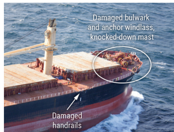
Figure 21. The damaged Ocean Princess after the casualty. BACKGROUND SOURCE: BUREAU OF SAFETY AND ENVIRONMENTAL ENFORCEMENT (ANNOTATED BY THE NTSB)
