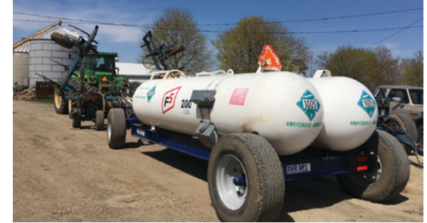
Figure 34. The farm tractor, fertilizer applicator, and nurse tank trailer involved in the anhydrous ammonia gas release in Beach Park, Illinois, that sent 83 people to the hospital. SOURCE: PHMSA
