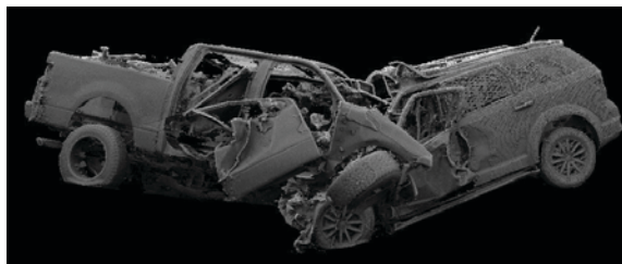
Figure 11. 3D point cloud data collected at the crash scene were analyzed to depict the interaction of the vehicles that collided in Avenal, California, where the SUV driver and all eight truck occupants died.
