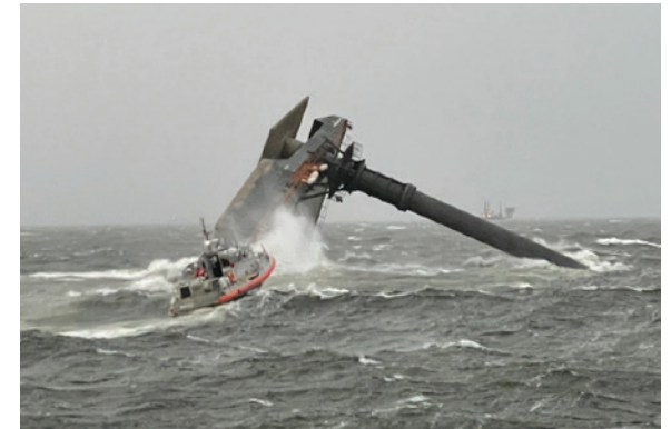
Figure 14. SEACOR Power capsized on its starboard side on the evening of the casualty. A US Coast Guard RB-M can be seen in the foreground. SOURCE: US COAST GUARD
