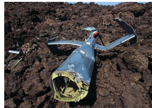
Figure 5. Separated helicopter tail boom on rough, lava rock-covered terrain at the accident site.
