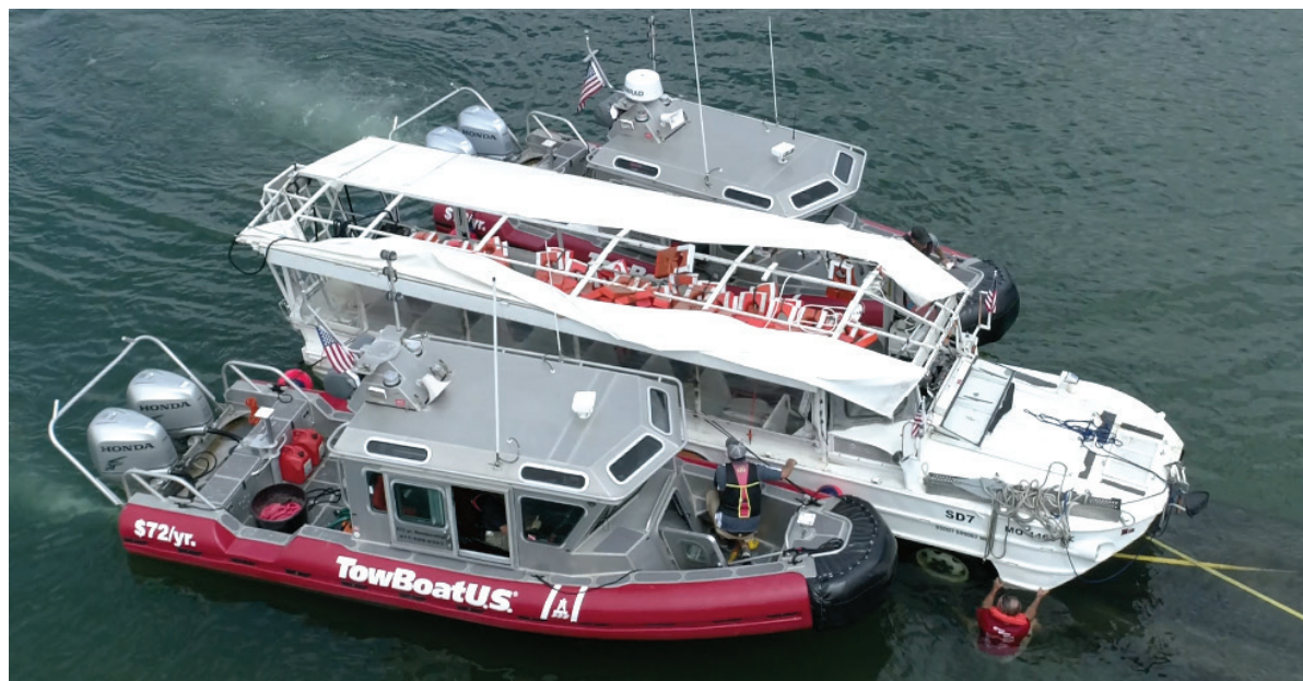
Figure 140. Torn canopy on the Stretch Duck 7 during recovery at Table Rock Lake.
