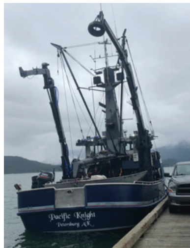
Figure 17. Left: the Pacific Knight while moored alongside a dock on June 10, 2018, with the two added cranes. Below: undated photo of the Pacific Knight (then named the Lone Fisherman ) with the aft deckhouse that was removed (highlighted in yellow). SOURCE: LONE FISHERMAN, LLC
