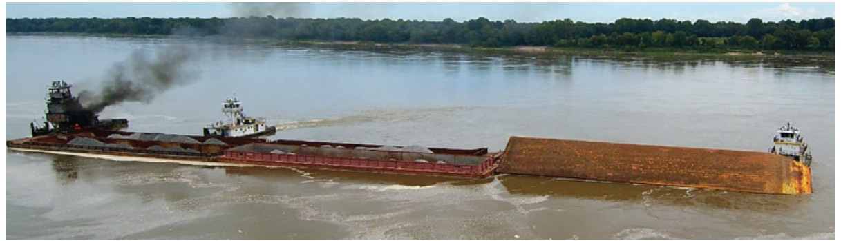
Figure 94. Two towing vessels push the remaining barges of the tow as the Jacob Kyle Rusthoven burns. The center head barge, which had turned over, sits on top of the port head barge. SOURCE: COAST GUARD
