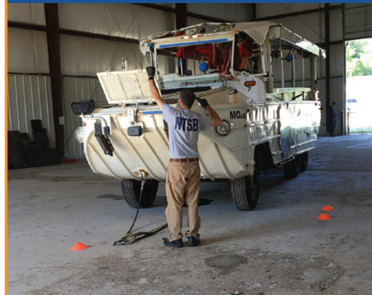
Figure 146. NTSB investigator inspecting the accident vessel's bow hatch.
