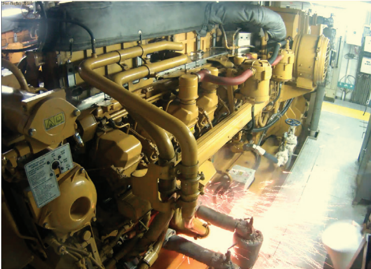
Figure 162. Screenshot from closed-circuit television at the time of the failure, looking aft from the inboard side of MDG no. 2.
