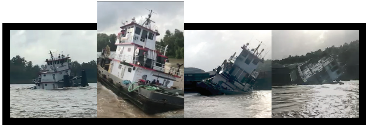
Figure 8. Sequence of events as the Miss Roslyn headed toward moored barges with a heavy list to starboard and eventually capsized. Left to right: (1) About 1650, the Miss Roslyn began crossing the Mississippi River with a noticeable list to starboard. As the vessel crossed the river, water increased on deck, and the vessel sank lower into the water. (2) The deckhands evacuate the Miss Roslyn . (3) About 1658, the vessel's list increases rapidly to starboard. (4) About 1659, the vessel lists further to about 90 degrees. SOURCE: CLAY HEBERT, ITV KRISTY DUTSCH
