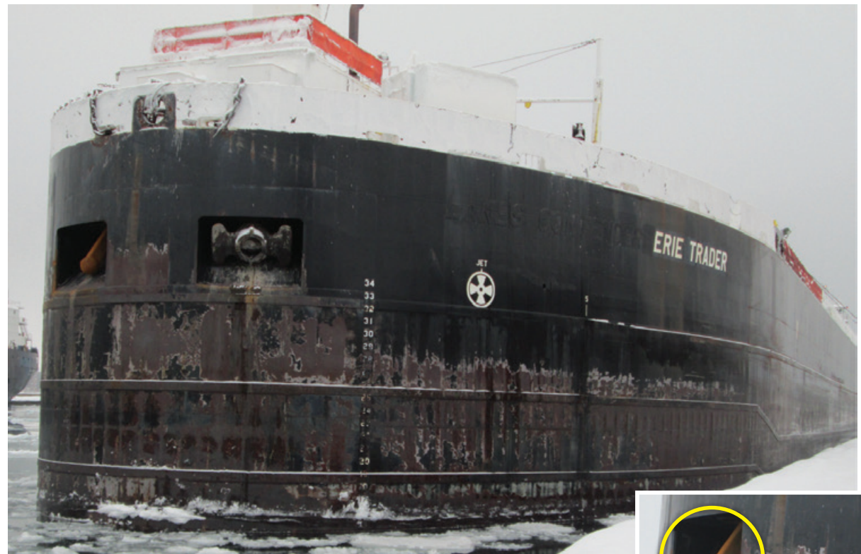
Figure 60. The bow of barge Erie Trader after the accident. At right: the remnant shank of the starboard anchor in the anchor pocket is highlighted. SOURCE: COAST GUARD
