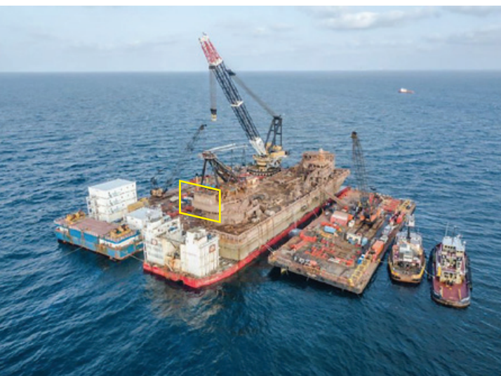
Figure 154. Left: Derrick barge TOPS DB1 loaded on BOABARGE 29 during offshore salvage operations in early 2018. Yellow outline highlights counterweight lifted by Atlantic Giant II .
