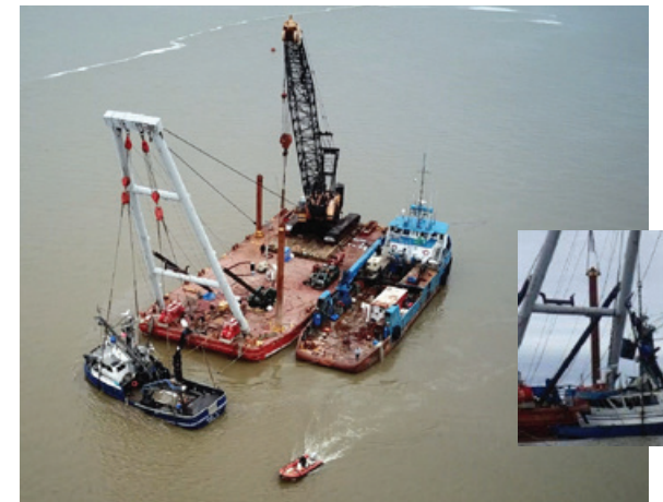
Figure 18. Pacific Knight while it was salvaged, with its crane positions visible in the inset.
