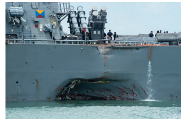
Figure 28. Portside damage to John S McCain caused by the bow of Alnic MC . SOURCE: US NAVY
