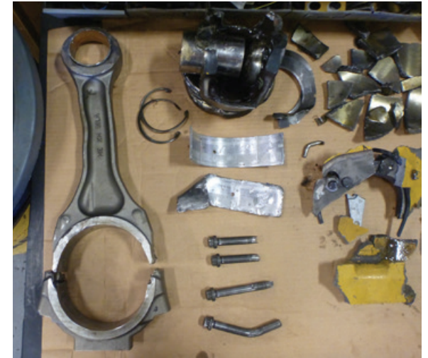
Figure 163. Connecting rod, cap, bolts, and bearing halves of cylinder no. 8. SOURCE: COAST GUARD
