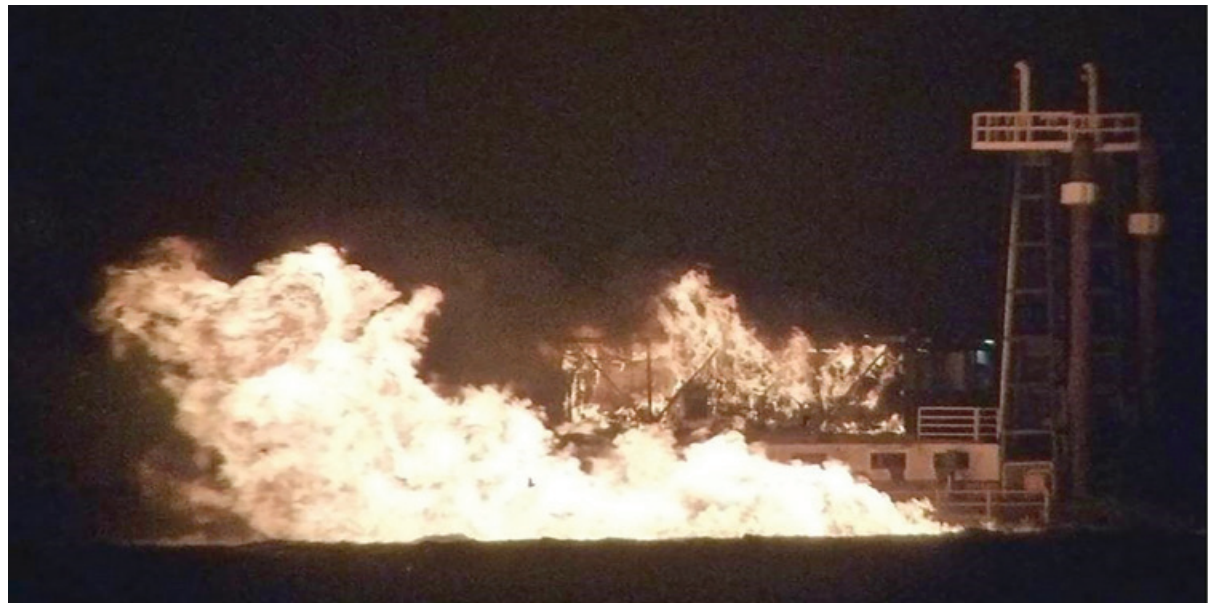
Figure 104. Jonathon King Boyd burns after striking a submarine gas pipeline.
