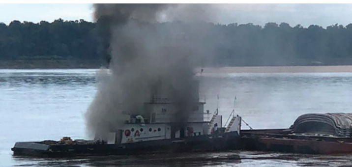
Figure 96. Smoke emanating from the open starboard-side and aft engine room doors on the main deck.
