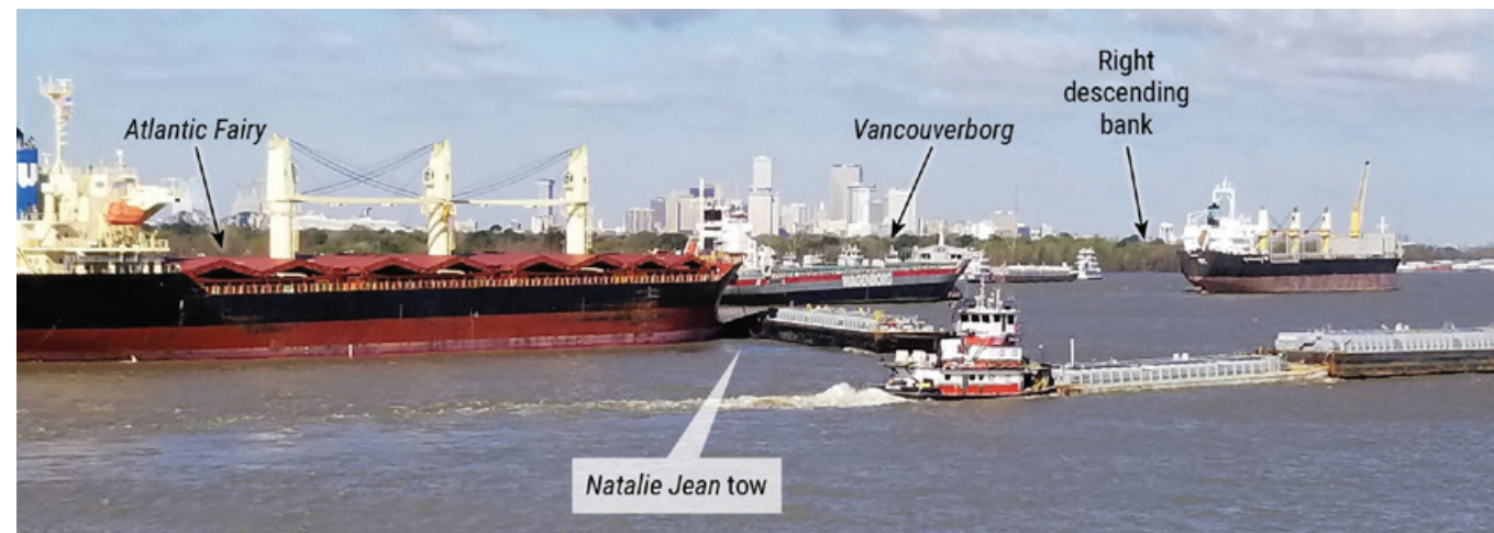
Figure 14. Photo (looking upriver) of the Natalie Jean tow perpendicular to the Atlantic Fairy . The towboat has capsized and is sinking. SOURCE: MORAN TOWING
