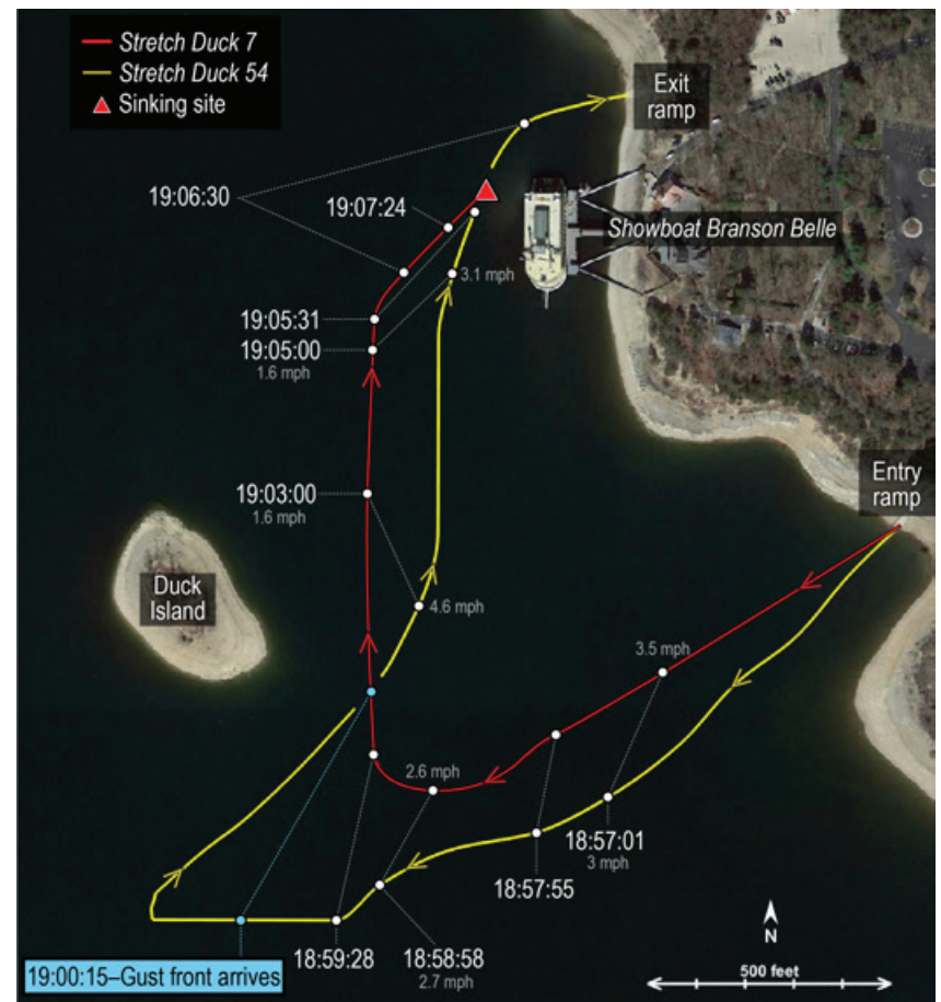
Figure 141. Vessel voyages on Table Rock Lake the evening of the accident. Red line represents the calculated trackline of the Stretch Duck 7 , and yellow line represents the actual trackline of the Stretch Duck 54 based on GPS data. 1
