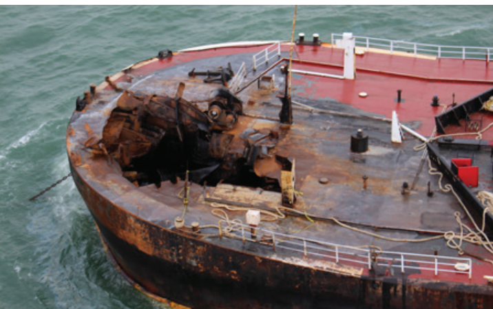
Figure 74. Explosion and fire damage to port bow of B. No. 255 . SOURCE: COAST GUARD
