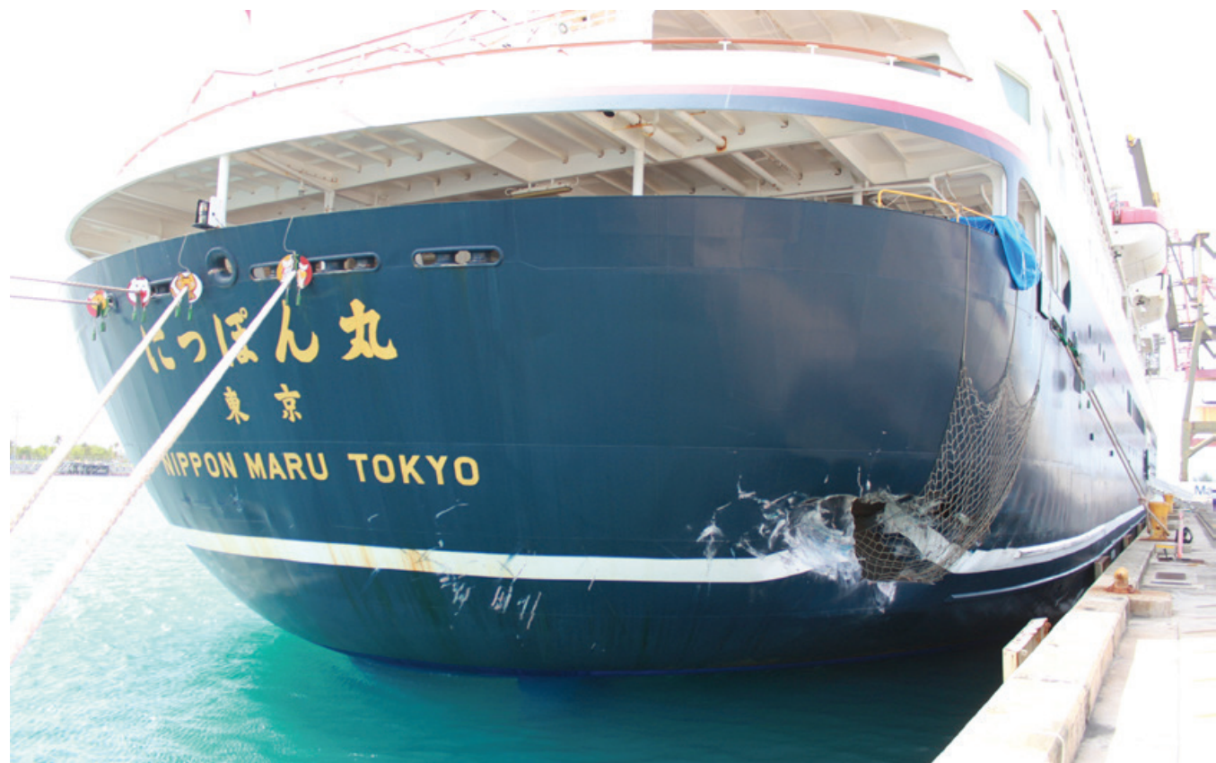
Figure 62. Starboard side of the stern of the Nippon Maru shows the damage to the ship.
