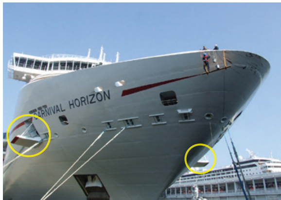
Figure 53. Carnival Horizon 's bow after the accident. The forward mooring platforms where the lookout was stationed (about a 100 feet aft from the tip of the bow) are circled in yellow. SOURCE: COAST GUARD
